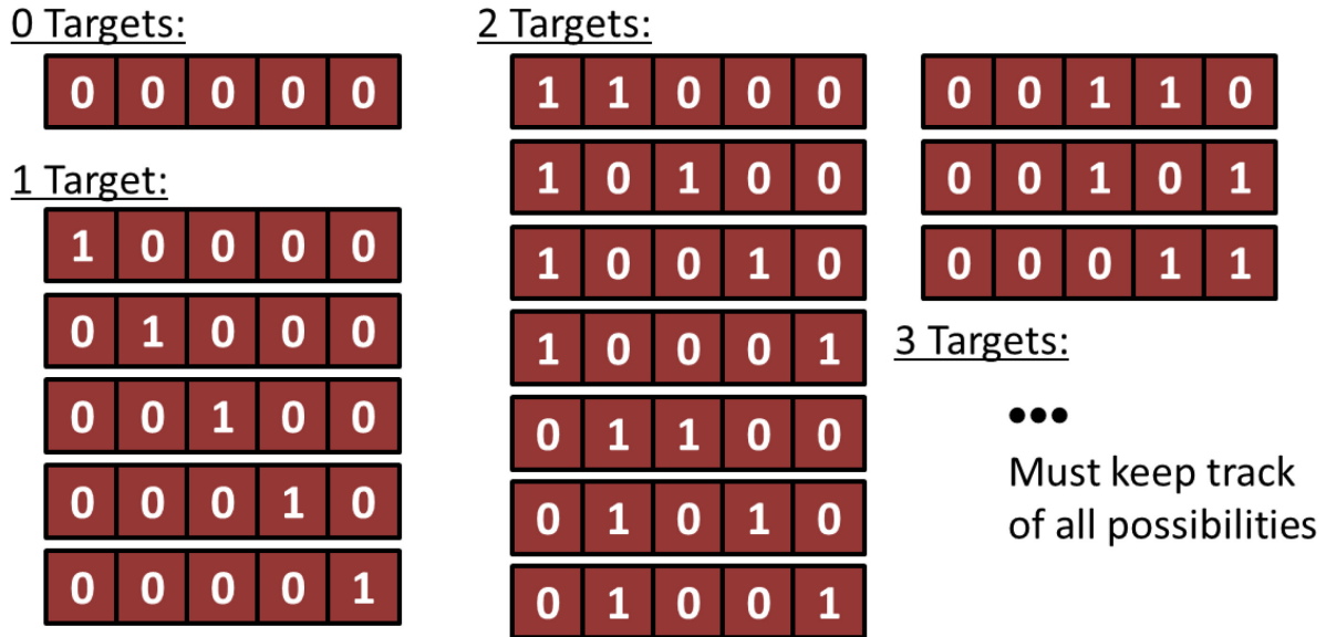
Figure 7: Depiction of different nuisance parameter combinations that can result from different number of targets present in the scene.
